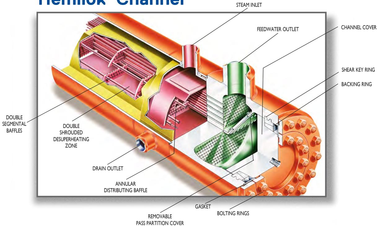
SPX Heat Transfer designs and manufactures both low pressure and high pressure feedwater heaters which may be installed either vertically or horizontally, depending on the plant design requirements. The physical and thermal characteristics are vastly different for high and low pressure feedwater heaters. Low pressure feedwater pressure ratings range between 400 and 800 psig, and high pressures range from 1,600 to 4,800 psig.
